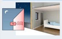
Night: Harvested heat is released from the buffer to inside of the building
