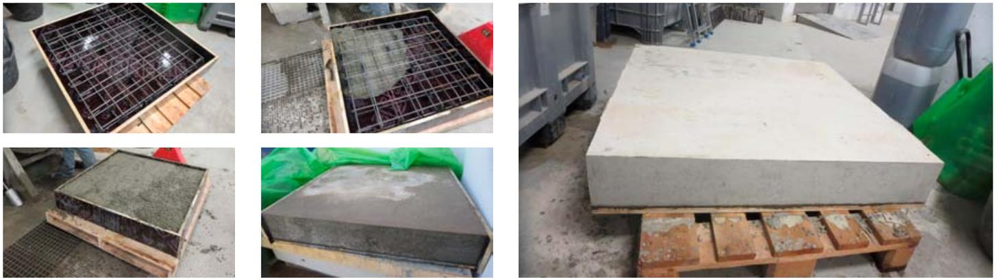
Figure: Preparation of a labscale prototype of the buffer component of Adaptiwall.
