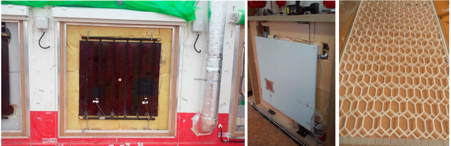
Figure 1: On the left: lab-scale prototypes of ADAPTIVALL, on the right: prototype of membrane separator.
